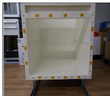
For non-adhesive gaskets, place small strips of double-sided tape on the flange(s).
