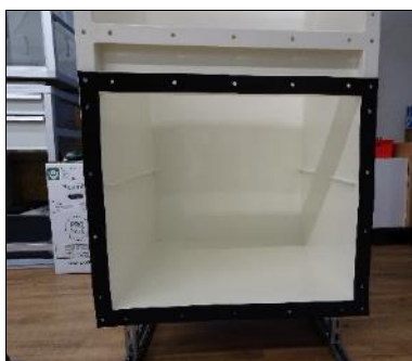
Place gasket(s) on the flange(s), aligning flange and gasket holes.
