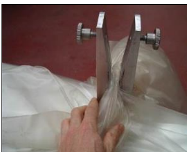
Slide the bag into the U-shape and insert the mobile part
