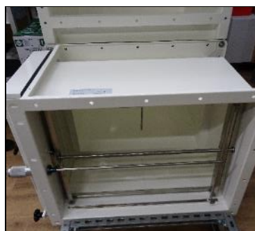
Place 1 st module, aligning flange holes.
